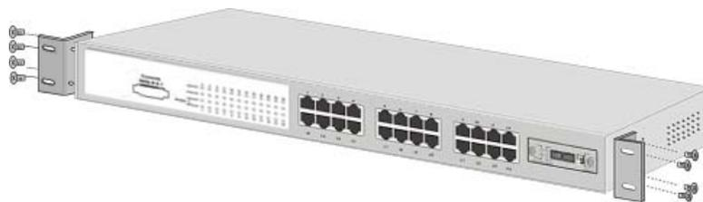
*Figure 2-4. Attach mounting brackets with screws*
