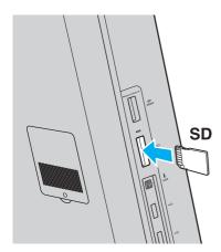
When you insert the SD memory card into the slot for the first time, you may be prompted to install driver software. If prompted, follow the on-screen instructions to install the software.
