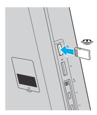
Before using "Memory Stick Micro" ("M2"), be sure to insert it into an "M2" Duo adaptor. If you insert the media directly into the "Memory Stick Duo" slot without the adaptor, you may not be able to remove it from the slot.
