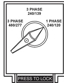
**Figure 28. Voltage Selector Switch 240/120V Single-Phase Position**
