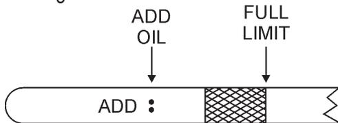
Figure 30. Engine Oil Dipstick
