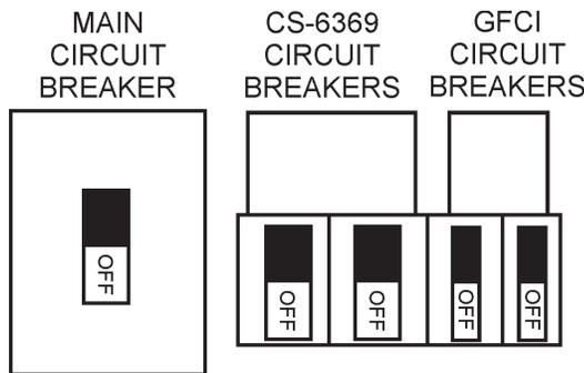
**Figure 38. Main, Aux. and GFCI Circuit Breakers (OFF)**
