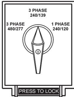
**Figure 21. Voltage Selector Switch 240/139V Three-Phase Position**
