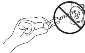
Backfeed to a utility system can cause **electrocution** and or property damage. **NEVER** connect the generators to a building's electrical system without a transfer switch or other approved device. All installations should be performed by a **licensed electrician** in accordance with all applicable laws and electrical codes. Failure to do so could result in electrical shock or burn causing serious injury or even death!
