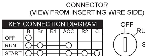
Figure 59A. Engine Wiring Diagram
