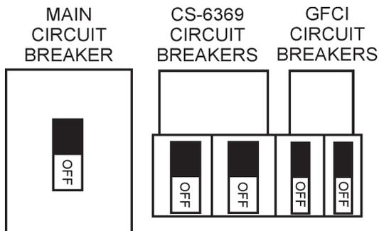
**Figure 53. Main, AUX. and GFCI Circuit Breakers (OFF)**
