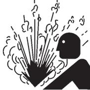
■ **Engine Oil Drain Plug** - Removing the engine oil drain plug while the engine is hot will result in hot oil gushing out of the oil drain plug, therefore causing severe scalding to any persons in the general area of the generator.
