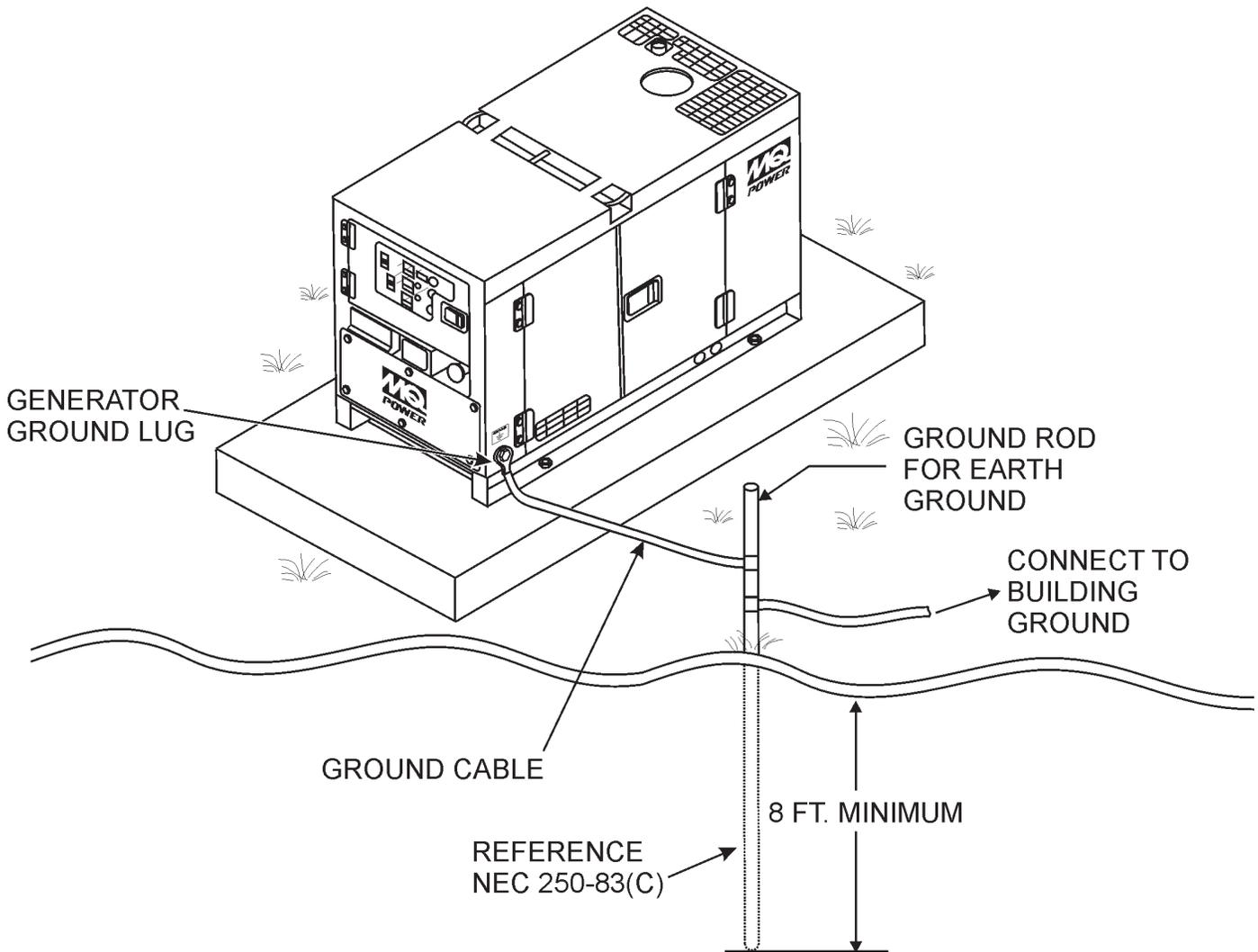
Figure 4. Typical Generator Grounding Application
