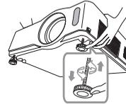
To finely adjust, twist the foot.
