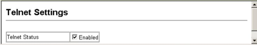
**CLI** – This example enables Telnet access to the switch.
