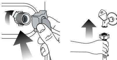
3. Open the taps completely after making the hose connection to check for water leaks at the connection points. If any leaks occur, turn off the tap and remove the nut. Retighten the nut carefully after checking the seal. To prevent water leakages and damages caused by them, keep the taps closed when the machine is not in use.
