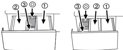
**i** The detergent dispenser may be in two different types according to the model of your machine as seen above.
