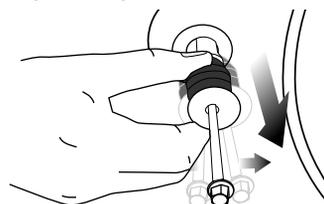
3. Attach the plastic covers supplied in the User Manual bag into the holes on the rear panel. (P)
