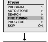
In FINE TUNING sub-menu, press P- or P+ to select TUNING, then press and hold V+ or V- to fine tune to obtain best possible picture and sound.
