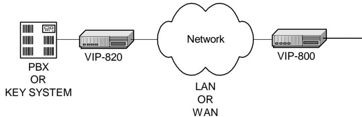
In this example, the VIP-810 and VIP-800 are connected to the data network as stand alone paging. This could be installed where network access is available, but not paging.
