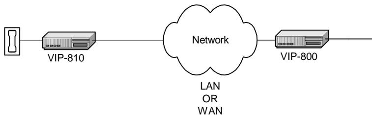
In these examples, two VIP-800's are connected to the data network to extend a paging zone to a remote location.
