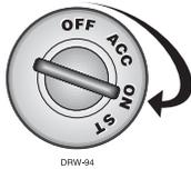
1. Insert the ignition key and turn it to the ON (not the START) position.
