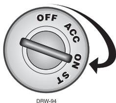
To override the starter kill, turn the ignition to the On position. Press the Valet button once within 10 seconds. The in-
