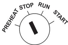
**Figure 71. Ignition Key Switch (STOP position)**
