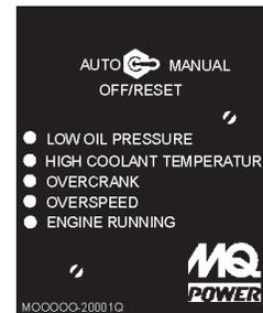
Figure 65. Engine Running LED (ON)
