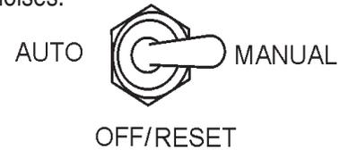
Figure 63. Auto-Off/Reset-Manual Switch
