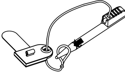
4. Slip the stylus into the elastic holder, and you're finished.
