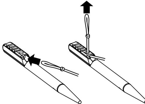
2. Thread the tether through the eyelet on the strap.
