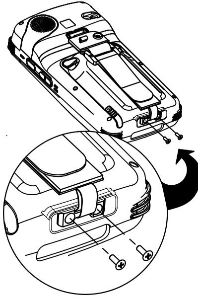
4. Adjust the handstrap by pulling up the Velcro tab and readjusting to your hand as needed.
