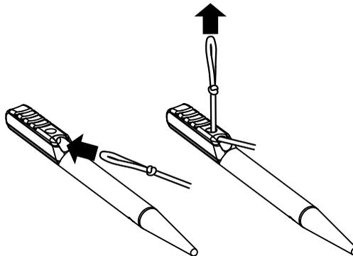
2. Thread the tether through the eyelet on the strap.
