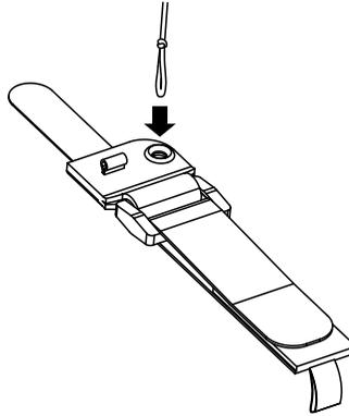
3. Pass the stylus through the tether loop and pull the tether snug.
