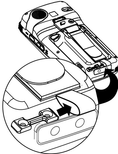
3. Slide the bracket through the plastic loop on the handstrap and install the screws.
