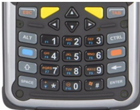
The [SHIFT], [CTRL] and [ALT] keys operate much like a desktop keyboard except that they are not chorded (two keys held down simultaneously). The modifier key must be pressed first followed by the key whose function you want modified.
