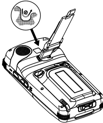
2. Remove the bracket and screws from the Ikôn.
