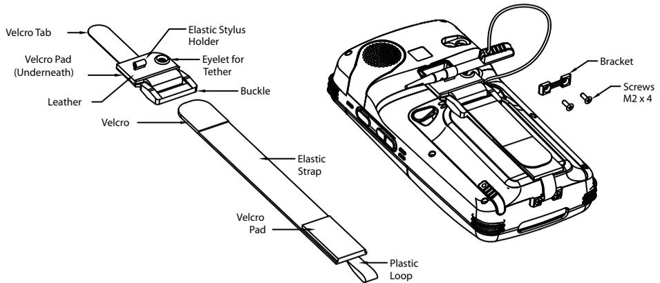
1. Attach the handstrap to the Ikôn by looping the Velcro tab around the pin and adhering the tab to the Velcro pad.
