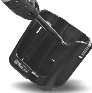
To accommodate the service loop of the power cable, leave a 10.2 cm (4 in.) clearance at the bottom of the vehicle cradle. Leave a 17.8 cm (7 in.) clearance at the top of the vehicle cradle to allow easy removal of the Ikôn. When selecting a mounting location, refer to the detailed assembly instructions that are packaged with the pedestal.
