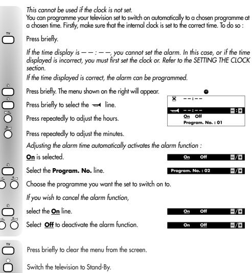
The Stand-By light flashes. The television will switch on to the selected channel at the time programmed. The symbol - appears on the bottom right of the screen. It will automatically switch off after five minutes if no key is pressed on the remote control or on the television keypad.
