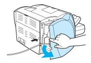
Pull out on the rear of the cover, and rotate it away from the printer.
