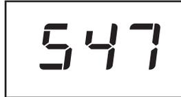
The Distance/Incline display will show the total number of miles (or kilometers) that the walking belt has moved.
