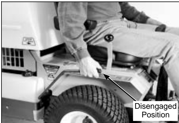
PTO Clutch Disengaged (Model MD Shown)
