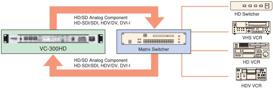
Figure 2. A multi-format converter is indispensable during post production, when many and varied video formats have to be dealt with. Used together with a matrix switcher, the VC-300HD can greatly boost efficiency and simplify conversion tasks from basic conversion to aspect ratio control, color adjustment, and other tweaks.
