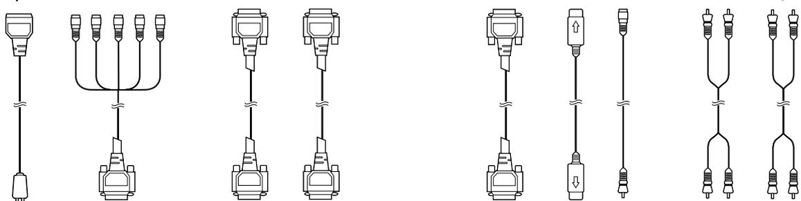
To receptacle    To color difference output terminal / To display (analog RGB) output terminal    To display (analog RGB) output terminal    To display (digital RGB) output terminal    To RS-232C output terminal    To S-video output terminal    To video output terminal    To sound output terminal    To sound output terminal
