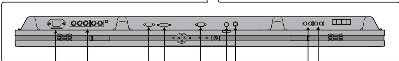
POWER INPUT    COMPONENT VIDEO INPUT (color difference input) / RGB3 INPUT    RGB2 INPUT (mD-sub)    RGB1 INPUT (DVI-D)    RS-232C    S-VIDEO INPUT    VIDEO INPUT    AUDIO2 INPUT    AUDIO1 INPUT
