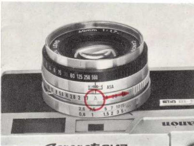
Turn the **automatic/manual** aperture ring, releasing it from "A" position, and set it for manual control of aperture. In this case, any **f/stop** can be set.
