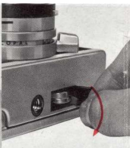
Before using your Canonet G-III, load it with the mercury battery.
