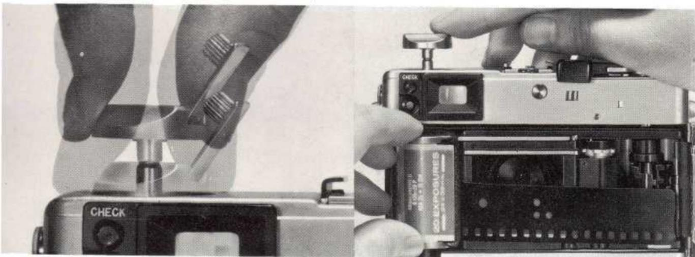
Canon's Exclusive Quick-Loading (QL) mechanism in the Canonet G-III accepts any standard 35mm film roll in cartridge. When loading new film, always avoid direct sunlight.
