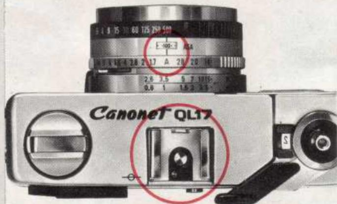
The Canolite D is an optional electronic flash unit with direct contact exclusively designed for the Canonet G-III. There is absolutely no necessity for worrying about guide numbers. Night or indoor photography is now as easy as daylight photography using the Canolite D.
