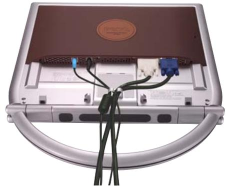
6. Put the back cover back and then separate the legs of the stand and place the monitor on a stable surface.
