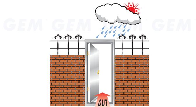
This series of Waterproof Magnetic Lock is made with epoxy potting compound and is protected by this compound. Also, GEM Waterproof Series Magnetic Locks have been proved to have withstood a water resistance as established in accordance with the test procedures of IPX7, IPX8 through a trusted third party. Therefore users need not worry that the lock will be rusted or sparked, if the lock is using in outdoor applications and installing in confined space where any inflammable gas.
