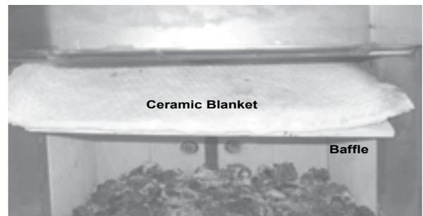
**Figure 20B - Baffle & Ceramic Blanket on top.**
