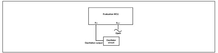
Figure 2.22 External oscillator circuit
