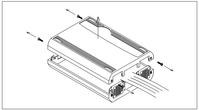
Figure 2.18 Removing the upper cover
