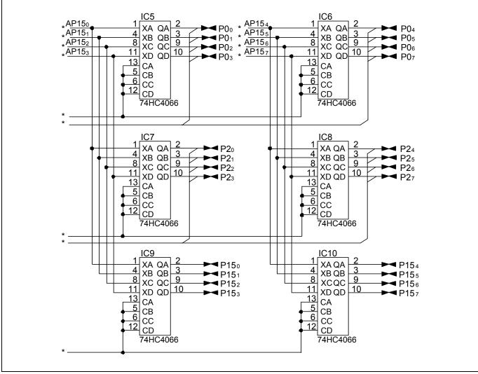
Figure 4.3 Connection diagram (3/3)
