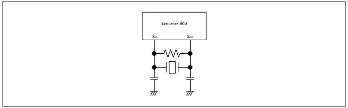
Figure 2.23 Circuit in which oscillation does not occur
