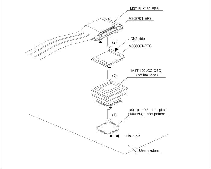
Figure 2.12 Connecting to a 100-pin 0.5-mm-pitch foot pattern (1/3)
