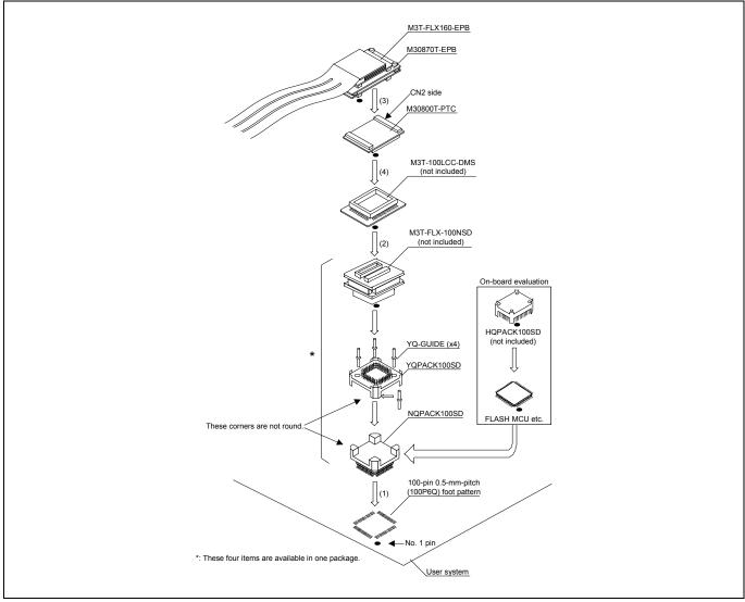
Figure 2.13 Connecting to a 100-pin 0.5-mm-pitch foot pattern (2/3)
