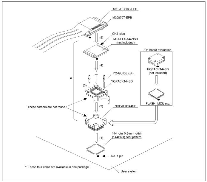
Figure 2.15 Connecting to a 144-pin 0.5-mm-pitch foot pattern
