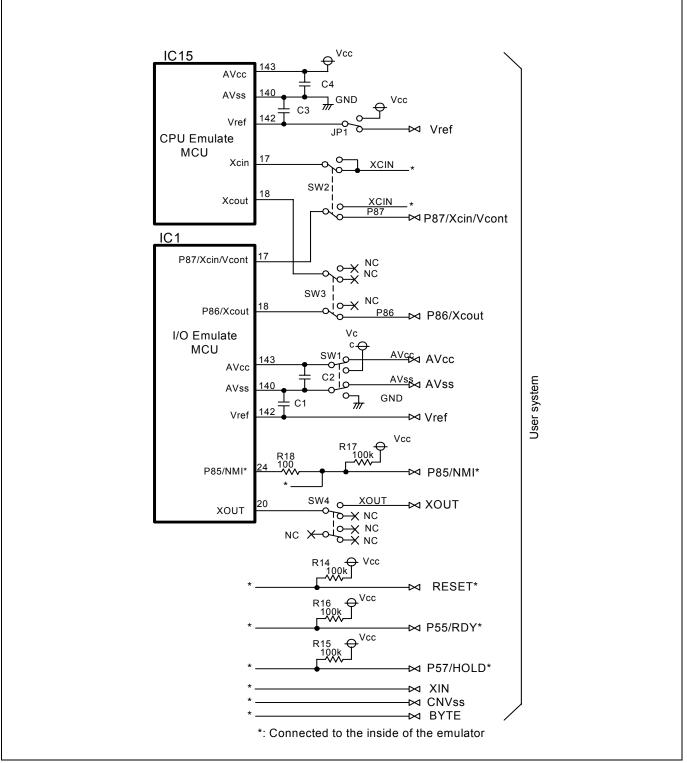
Figure 4.2 Connection diagram (when using M30870T-EPBM REV.C) (2/3)
