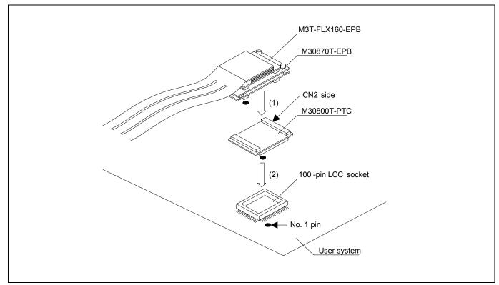
Figure 2.8 Connecting to a 100-pin LCC socket
