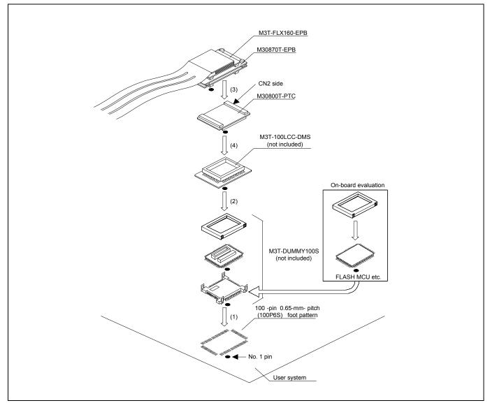
Figure 2.9 Connecting to a 100-pin 0.65-mm-pitch foot pattern (1/3)
