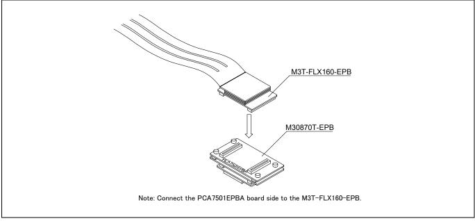
Figure 2.3 Connecting the PC7501 and emulation probe
