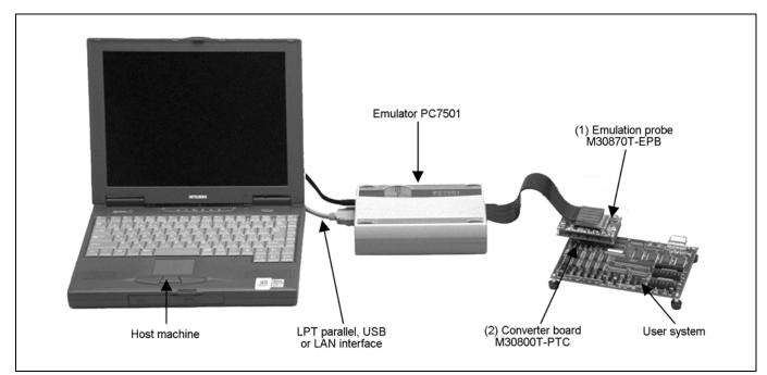
Figure 1.1 System configuration
