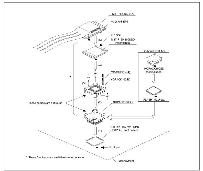
Figure 2.14 Connecting to a 100-pin 0.5-mm-pitch foot pattern (3/3)
