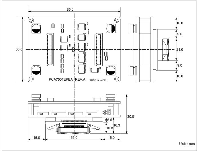
Figure 4.4 External dimensions of the emulation probe
