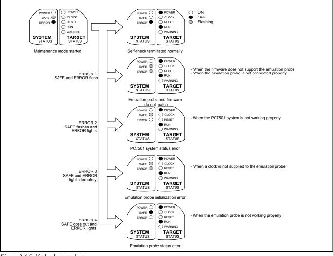
Figure 2.6 Self-check procedure
