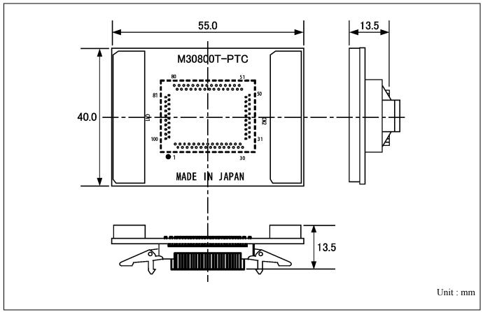
Figure 4.5 External dimensions of the M30800T-PTC
