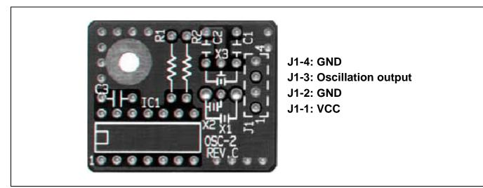
Figure 2.20 External view of the oscillator board OSC-2 (bare board) and connector pin assignments
