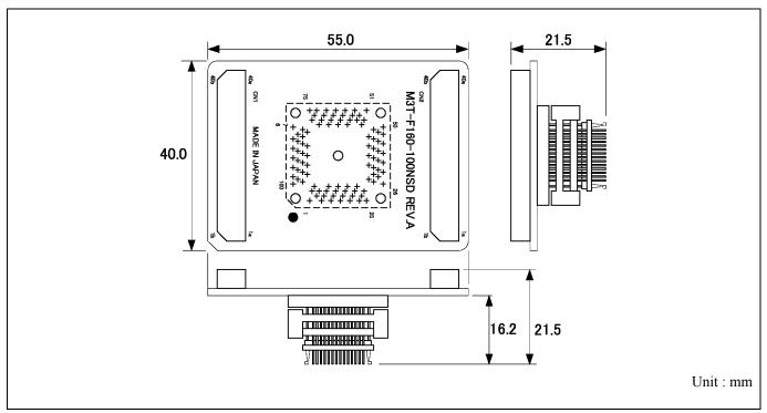
Figure 4.6 External dimensions of the M3T-F160-100NSD
