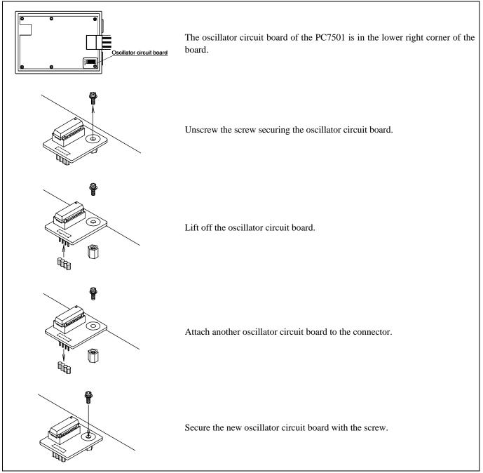
Figure 2.19 Replacing oscillator circuit boards
