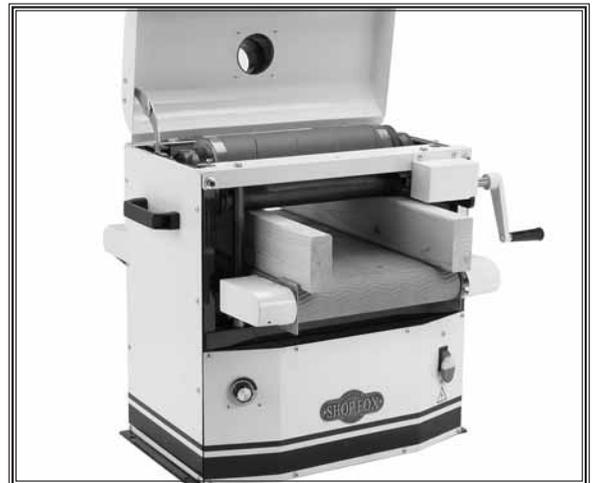
**Figure 30.** Gauge boards in position.
