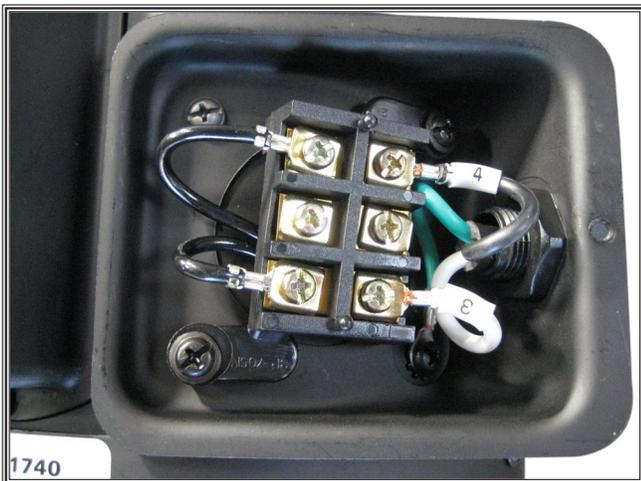
Figure 6. Drum motor wiring.
