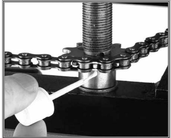
**Figure 40.** Marking sprocket and lead screw timing.
