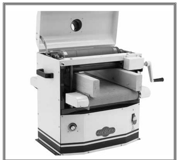
**Figure 27.** Gauge boards in position.
