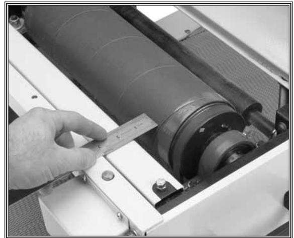
**Figure 33.** Measuring drum alignment.
