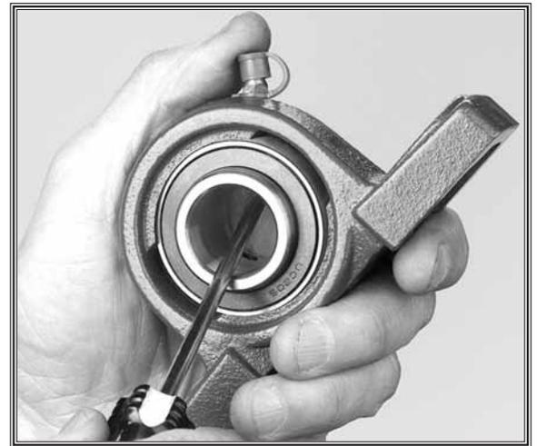
Figure 56. Bearing positioning for removal.
