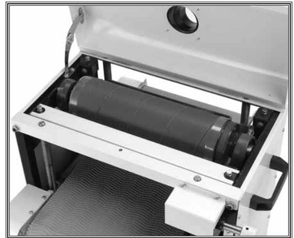
**Figure 13.** Sandpaper installed and taped.
