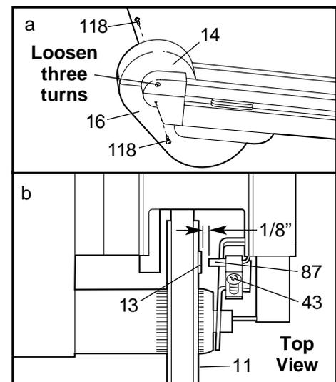
**PROBLEM: The grade of the hiker does not change correctly or does not change when iFit.com CD's and videocassettes are played**
