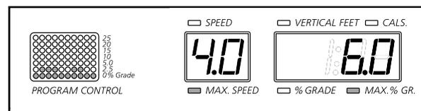
longest programs, the matrix will not show all of the grade settings at once.) In addition, the Speed display will show the maximum speed setting for the program and the Vertical Feet/Cals./Grade display will show the maximum grade setting for the program.
