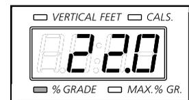
**The Distance/Time display**—When the manual mode or an iFit.com program is selected, this display will show the distance you have hiked and the elapsed time. The distance will be shown for seven seconds and the time will be shown for fourteen seconds, as shown by the indicators around the display.
