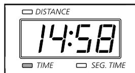
When a preset program is selected, the Distance/Time display will show the distance you have hiked, the time remaining in the program, and the time remaining in the current segment of the program.
