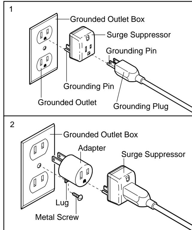
The temporary adapter should be used only until a properly grounded outlet (drawing 1) can be installed by a qualified electrician.
