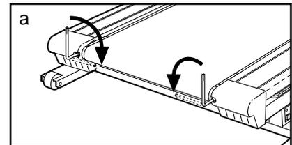
b. **If the walking belt has shifted to the right**, first remove the key and **UNPLUG THE POWER CORD**. Using the allen wrench, turn the left rear roller adjustment bolt counterclockwise, and the right bolt clockwise, 1/4 of a turn each. Be careful not to overtighten the walking belt. Plug in the power cord, insert the key and run the hiker for a few minutes. Repeat until the walking belt is centered.
