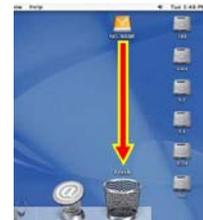
Eject the volume before powering down the unit by dragging the volume's icon to the trash bin, or by selecting the volume then pressing Command-E.
