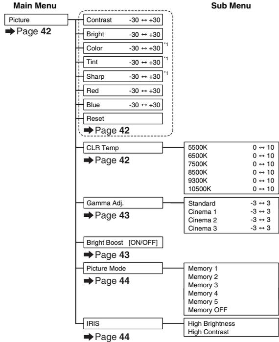
\*1: Items when selecting INPUT 1, 2, 3, 4 or when inputting component signal through INPUT 5
