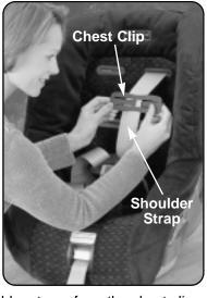
Remove the shoulder straps from the chest clip on the front of the car seat.
