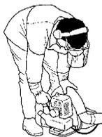
**WARNING:** When starting engine, hold the unit as illustrated. Do not set unit on any surface except a clean, hard area when starting engine or while engine is running. Debris such as gravel, sand, dust, grass, etc. could be picked up by the air intake and thrown out through the discharge opening, damaging the unit or property, or causing serious injury to bystanders or the operator.
