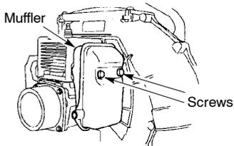
3. Remove the spark arresting screen.
