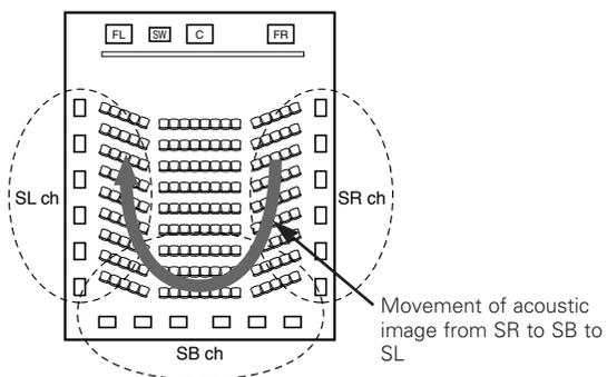
In addition to sources recorded in 6.1-channels, the surround effect of conventional 2- to 5.1-channel sources can also be enhanced.
