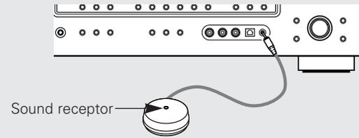
**2** Mount the setup microphone on a camera tripod, etc., and set with the receptor pointing towards the ceiling.
