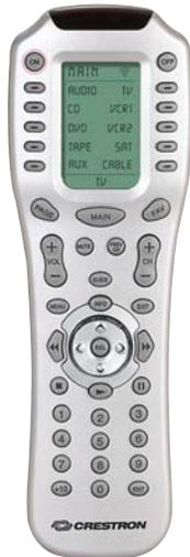
The ML-600 MiniLCD is a handheld wireless remote that features a customizable LCD display, a 5-way thumb pad controller, and an intuitive array of pushbuttons designated for a variety of common AV functions. But Crestron designed the ML-600 to go beyond conventional home theater and AV system control, extending domain over lighting, climate, security, and more as part of a complete Crestron system. Its compact size and ergonomic design offer easy one-handed operation.
