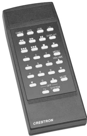
The CNRFHT wireless handheld remotes communicate via 1-way RF with any Crestron control system using the CNRFGWA RF gateway, or the RF gateway built into the MC2W wireless control system. Two models are available, the CNRFHT-30A and the CNRFHT-15A.
