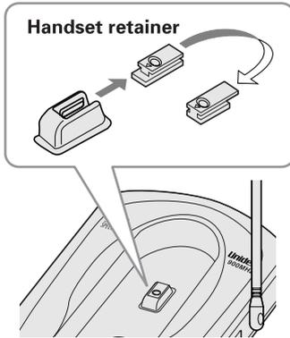
**8** On the base unit, pull the handset retainer out of the slot. Rotate it clockwise 180 degrees.
