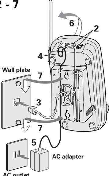
2 Plug the telephone line cord to the **TEL LINE** jack and the AC adapter to the **DC IN 9V** jack.
