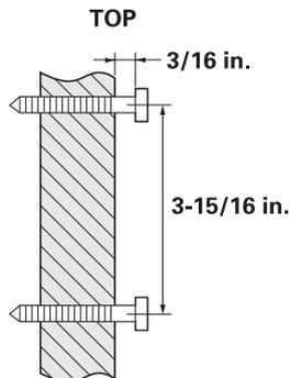
**1** Insert two mounting screws into the wall, (with their appropriate anchoring device), 3-15/16 inches apart. Allow about 3/16 of an inch between the wall and screwheads for mounting the phone.
