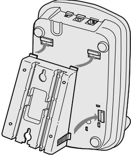
1 Snap the wall mount adapter into the notches on the base.
