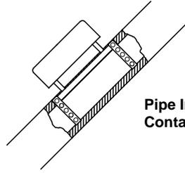
Pipe Insulation Should Cover Shield Containing Element.
