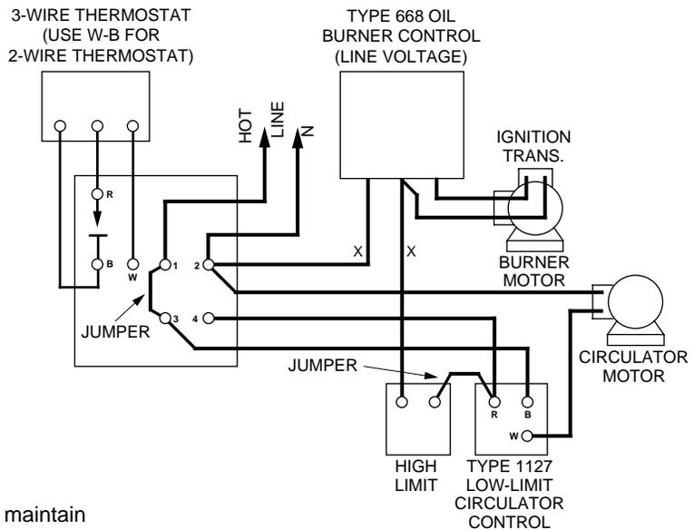
The R-B contacts of the low-limit circulator control maintain domestic hot water at the desired temperature year-round.
