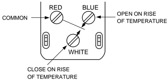
This control has a single-pole, double-throw snap action switch. The top left-hand terminal (red) is the common terminal. The top right-hand terminal (blue) has open-on-rise switch action. The bottom centre terminal (white) has close-on-rise switch action.
