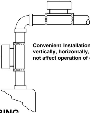
Convenient Installation – May be mounted vertically, horizontally, or on an angle. Will not affect operation of control.
