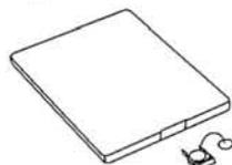
Insert battery holder into controller.
