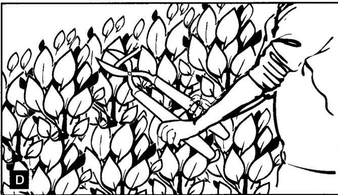
Do not attempt to cut branches thicker than 16 mm (0.6") diameter with this trimmer. These should first be cut with shears (fig. D) down to the hedge trimmer level.
