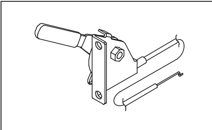
Speed control lever assembly for Vanguard™ V-Twin horizontal crankshaft models.
