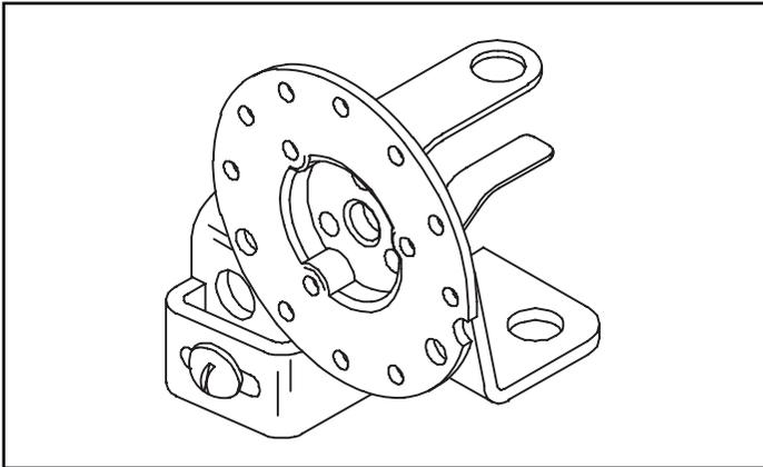
Disc type throttle control allows for remote speed operation.
