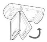
Push the monitor back into its main unit so that the screen clips back into the releasing/locking mechanism
