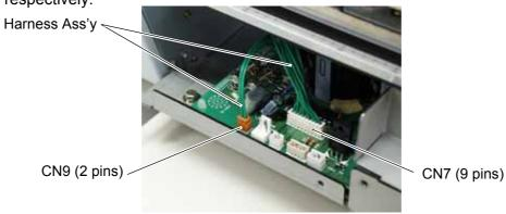
22) Fit the bush to the harness ass'y in the orientation as shown below.
