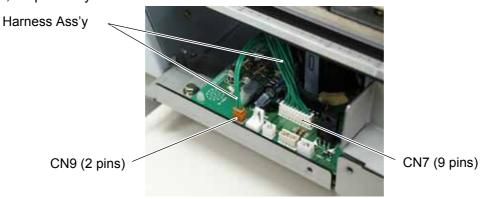
9) Fit the bush to the harness ass'y in the orientation as shown below.
