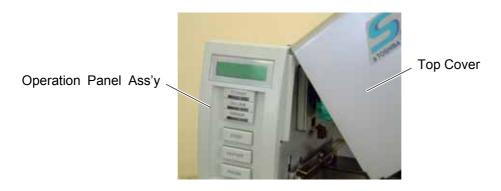
Lift the operation panel ass'y to release the hook, and then remove the operation panel ass'y by moving it forward. 10) Disconnect the operation panel harness from the operation panel ass'y.
