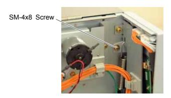
8) Half open the top cover, otherwise the operation panel ass'y cannot be removed from the printer.
