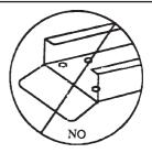
▲WARNING! In the following assembly process, the flange pictured must face down with the Tongue (10) edge fully contacting the tailgate. It is designed to keep the Ramps from moving once the weight of the load is riding on the ramp.
