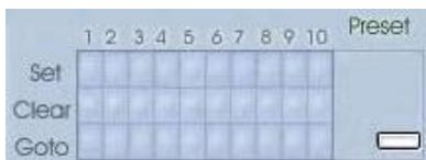
Each of the ten buttons under 'Set' is connected with a specific position and angle of either panning or tilting of the camera. Click each button to activate its particular position and angle. Press the button under 'Preset' to turn the camera angle by angle in the set positions.
