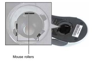
Replace the mouse ball and lock the retaining ring into place.
