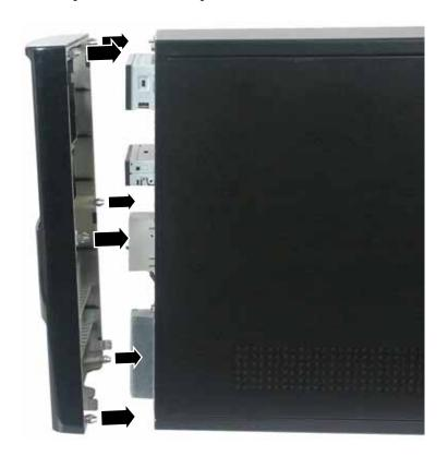
**2** Press the bezel firmly into place.
