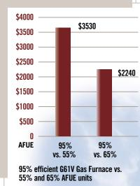
This chart depicts potential energy savings you can expect from the G61V furnace, versus older furnaces with lower efficiency ratings. Criteria used in this example are 2,000 full-load heating hours, with a 60,000 Btuh heating design load and \$1.281 ccf for gas. Your actual savings may vary, depending on the weather patterns in your local area, local fuel rates and your individual lifestyle.
