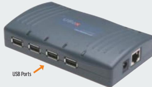
Above each USB port is a green LED light. This light indicates whether your USB device is supported in the current software/firmware. A solid green light indicates that your device is supported. A slowly blinking light indicates that your USB device is not currently supported. Please contact Lantronix if you have a slowly blinking light.
