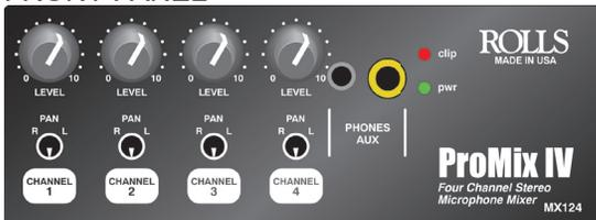
Mic Level 1 - 4: These controls adjust the level of the corresponding Mic channel. The level varies from -infinity (off) to max gain.
