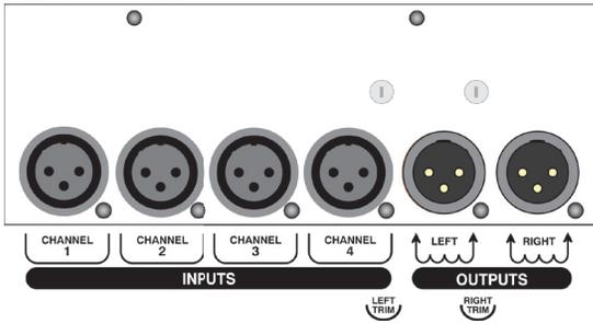
Mic Input: 1 - 4: XLR balanced inputs for connection to any standard dynamic or condenser microphone.
