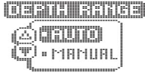
The 105SX automatically adjusts the depth range depending on the depth of the water. The unit tries to maintain the bottom depiction about  $\frac{2}{3}$  down the total range (for example, in 20' (6m) of water, the 0-30' (0-10m) range would be selected). This provides the best display resolution and therefore the best target separation possible.
