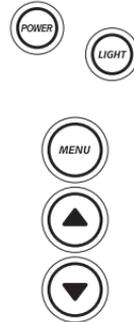
**Power.** The Power button powers the 105SX up for normal operation. When the unit is on, POWER turns the unit off. POWER can also be used to go directly into Simulator mode. To enter simulator, with the unit powered off, press and hold POWER for several seconds until a continuous chirp is heard.
