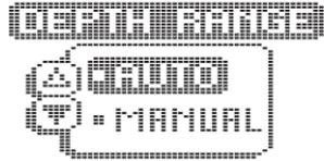
Within the menu are the options available. The selected option or current setting is highlighted in the black box. If no adjustment is made, this is the selected setting. Press an ARROW button while the menu is displayed to select another option.
