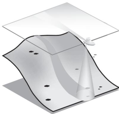
Sonar is very fast. A sound wave can travel from the surface to a depth of 600' (185m) and back again in less than  $\frac{1}{4}$  of a second. It is unlikely that your boat can "outrun" this sonar signal.
