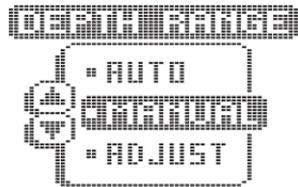
The Depth Range can be adjusted manually. Press MENU repeatedly until the Depth Range menu is visible. Two options are available: Auto and Manual.
