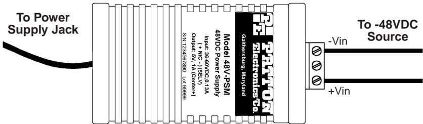
Figure 11. Connecting DC power to the 48V-PSM DC power supply
