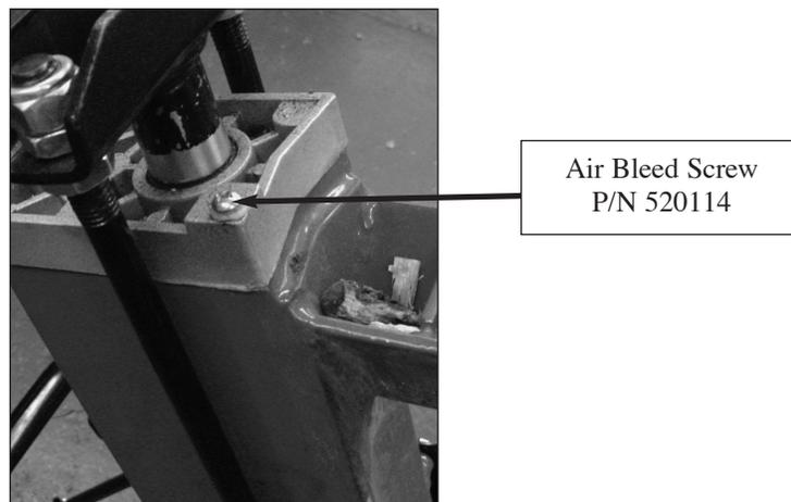
**NOTE: DO NOT OVER TIGHTEN AND STRIP AIR BLEED SCREW THREADS**
