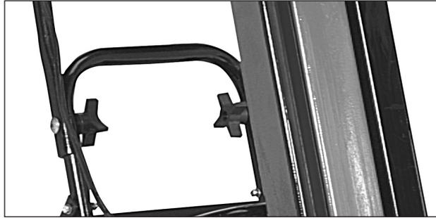
5. Use cable ties (P/N 520117) to secure the power cord in place.
