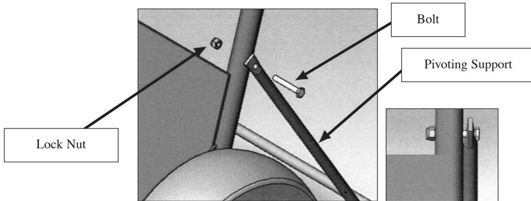
8. Attach Connecting Link (P/N 520105) to the Pivoting Support (P/N 520104).
