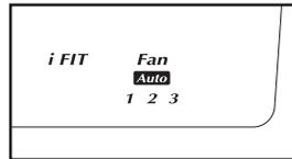
To turn off the fan, press the Auto Breeze Fan button again. Note: If the fan is left on when the walking belt is stopped, the fan will automatically turn off after a few minutes.
