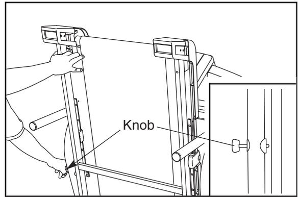
2. **Hold the metal frame firmly with both hands**, and lower the treadmill to the floor. **CAUTION: To decrease the possibility of injury, do not lower the treadmill by gripping only the plastic foot rails. Do not drop the treadmill frame to the floor. Be sure to bend your legs and keep your back straight.**
