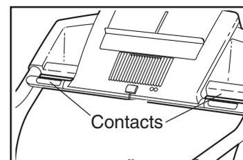
To measure your heart rate, **stand on the foot rails** and hold the metal contacts—**avoid moving your hands**. When your pulse is detected, the heart symbol beside the Pulse/Speed display will flash, one or two dashes will appear, and then your heart rate will be shown. **For the most accurate heart rate reading, continue to hold the contacts for about 15 seconds.**
