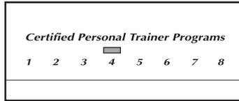
As each preset program is selected, the maximum speed setting of the program and the maximum incline setting of the program will flash in the displays for a few seconds. The Time/Pace display will show how long the program will last. A profile of the speed settings of the program will scroll across the matrix.
