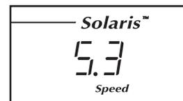
If one of the speed buttons numbered 1 through 10 is pressed, the walking belt will gradually increase in speed until it reaches the selected speed setting.
