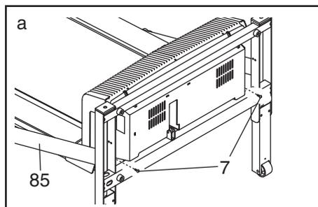
b. Raise the Uprights (85) to the vertical position. Remove the three 3/4" Screws (7) from the Hood (33), and carefully pivot the Hood off.
