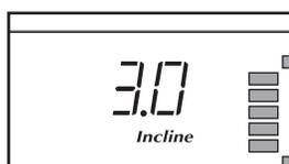
and the incline level of the treadmill. Note: Each time the incline changes, the display will show the incline setting.
