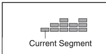
(The incline settings are not shown in the matrix.) The speed settings for the next few segments will be shown in the columns to the right.
