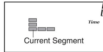
The speed setting for the first segment will be shown in the flashing Current Segment column of the matrix. (The incline settings are not shown in the matrix.) To program a speed setting and an incline setting for the first segment, simply adjust the speed and incline of the treadmill as desired by pressing the Speed and Incline buttons. Every few times a Speed button is pressed, an additional indicator will appear or disappear in the Current Segment column.
