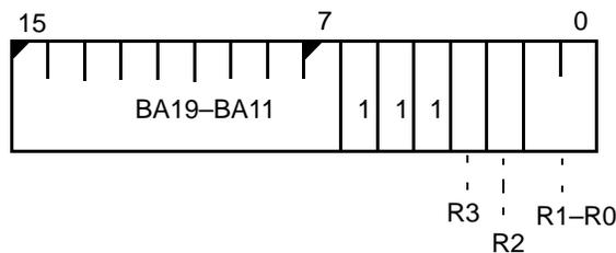
The value of the PACS Register at reset is undefined.
