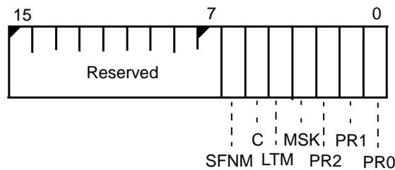
The value of IOCON and I1CON at reset is 000Fh.
