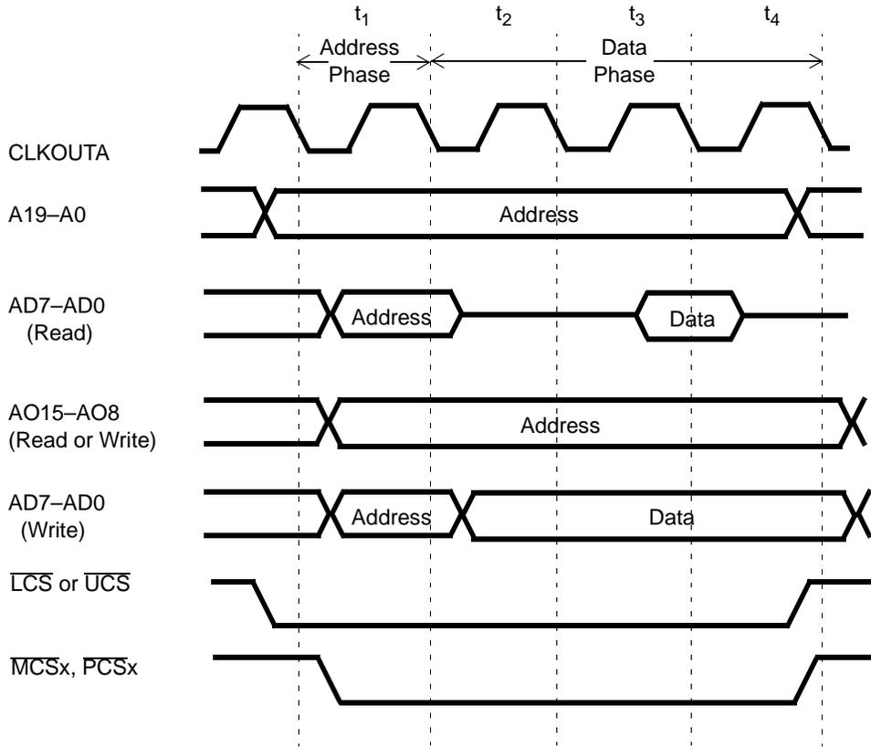
Figure 3-4 Am188ER Microcontroller—Read and Write with Address Bus Disable In Effect
