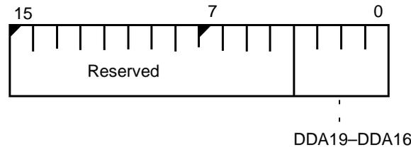
The value of D0DSTH and D1DSTH at reset is undefined.
