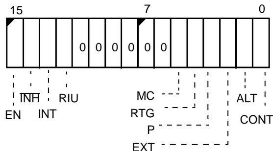
The value of T0CON and T1CON at reset is 0000h.
