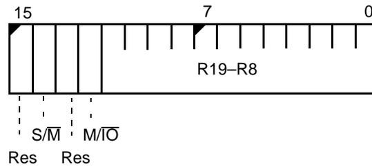
The value of the RELREG Register is 20FFh at reset.
