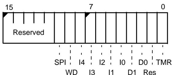
The INSERTV Register is set to 0000h on reset.
