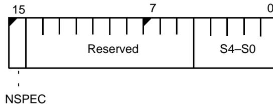
**Bit 15: Non-Specific EOI (NSPEC)**—The NSPEC bit determines the type of EOI command. When written as a 1, NSPEC indicates non-specific EOI. When written as a 0, NSPEC indicates the specific EOI interrupt type is in S4–S0.
