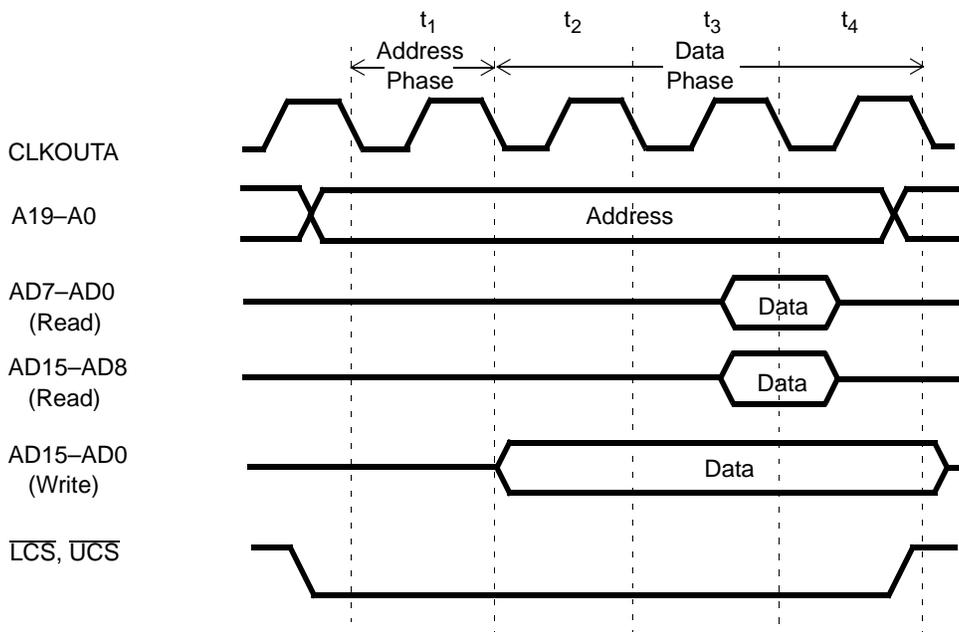
Figure 3-3 Am188ER Microcontroller Address Bus—Normal Read and Write Operation
