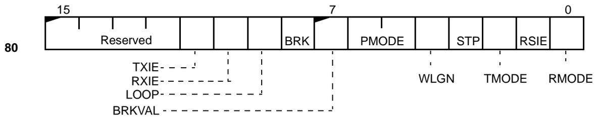
**Serial Port Control Register (SPCT)**
