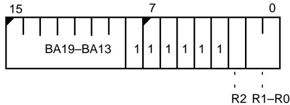
The value of the MMCS Register at reset is undefined.
