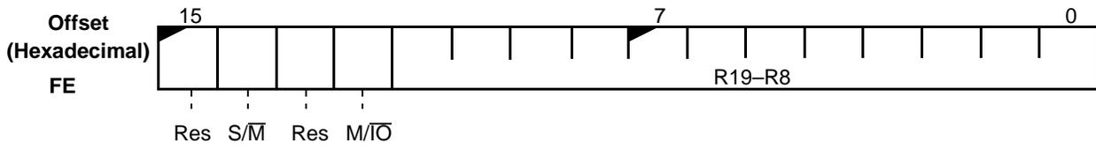
**Peripheral Control Block Relocation Register (RELREG)**
