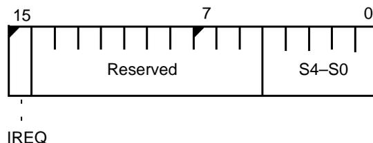
**Bit 15: Interrupt Request (IREQ)**—Set to 1 if an interrupt is pending. When this bit is set to 1, the S4–S0 field contains valid data.
