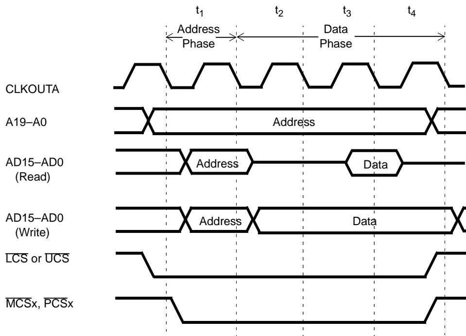
Figure 3-2 Am186ER Microcontroller—Read and Write with Address Bus Disable In Effect
