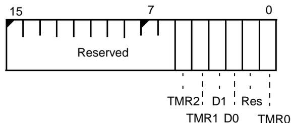
The IMASK Register is set to 003Dh on reset.
