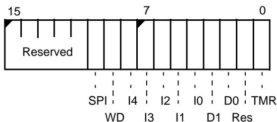
The IMASK Register is set to 07FDh on reset.
