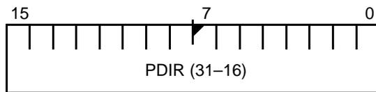
Figure 13-5 PIO Direction 0 Register (PDIR0, offset 72h)
