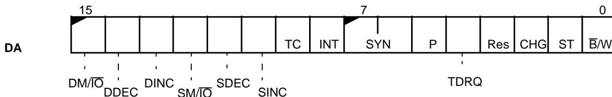
**DMA 1 Control Register (D1CON)**
