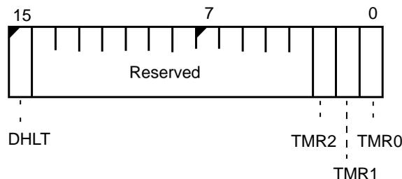
**Bit 15: DMA Halt (DHLT)**—When set to 1, halts any DMA activity. This bit is automatically set to 1 when nonmaskable interrupts occur and is reset when an IRET instruction is executed. Time-critical software, such as interrupt handlers, can modify this bit directly to inhibit DMA transfers. Because of the function of this register as an interrupt request register for the timers, the DHLT bit should not be modified by software when timer interrupts are enabled.
