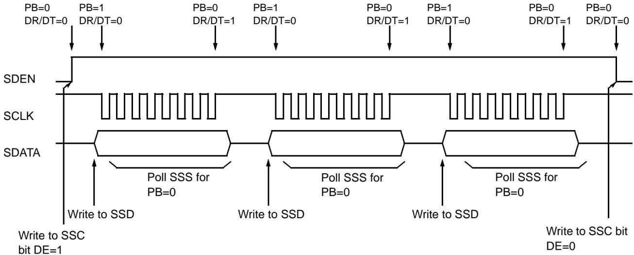
Figure 12-6 Synchronous Serial Interface Multiple Read
