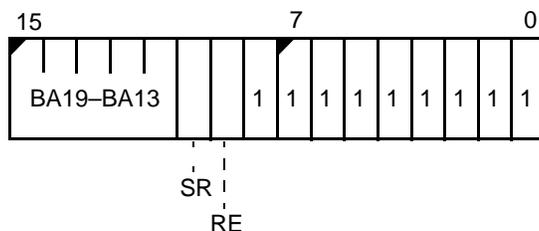
**Bits 15–11: Base Address (BA19–BA15)**—The base address of the internal RAM is determined by the value of BA19–BA15, which corresponds to bits A19–A15 of the 20-bit memory address. The base address can only be set on a 32-Kbyte boundary. The value of this field is undefined after processor reset.
