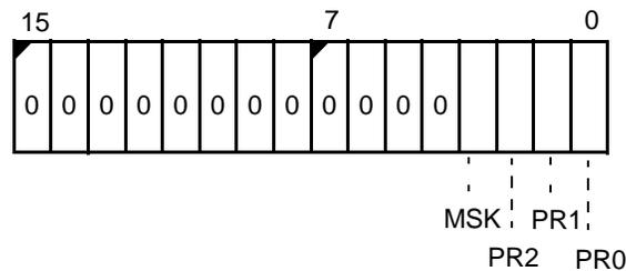
The value of TCUCON, DMA0CON, and DMA1CON at reset is 000Fh.
