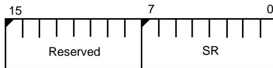
The value of this register at reset is undefined.
