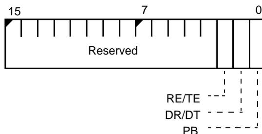
The value of the SSS register at reset is 0000h.
