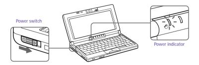
If you hold the power switch in the On position for more than four seconds, the computer turns off.
