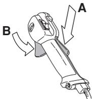
Make sure the throttle control is locked at the idle setting when the throttle lockout is released.
