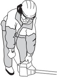
**CAUTION!** Do not put any part of your body in marked area. Contact can result in burns to the skin, or electrical shock if the spark plug cap has been damaged. Always use gloves. Do not use a machine with damaged spark plug cap.
