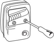
If the muffler on your machine is fitted with a spark arrestor screen this must be cleaned regularly. A blocked screen will cause the engine to overheat and may lead to serious damage.
