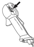
Start the engine and make sure the engine stops when you move the stop switch to the stop setting.
