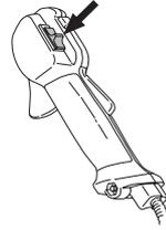
**CAUTION!** The stop switch automatically returns to the start position. In order to prevent unintentional starting, the spark plug cap must be removed from the spark plug when assembling, checking and/or performing maintenance.
