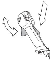
See instructions under the heading Start. Start the machine and apply full throttle. Release the throttle and check that the cutting attachment stops and remains at a standstill. If the cutting attachment rotates with the throttle in the idle position then the carburettor idle setting must be checked. See instructions under the heading Maintenance.
