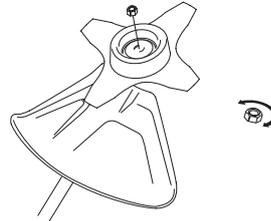
When loosening and tightening the saw blade nut, there is a risk of injury from the teeth of the saw blade. You should therefore always ensure that your hand is shielded by the blade guard when doing this. Always use a socket spanner with a shaft that is long enough to allow this. The arrow in the diagram shows the area where you should operate the socket spanner when loosening or tightening the nut.
